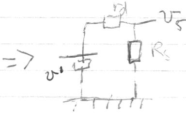
$$v_s = \frac{v_s' \cdot R_s}{R_s + r_d} = g_m v_{gs} \frac{r_d R_s}{R_s + r_d}$$
